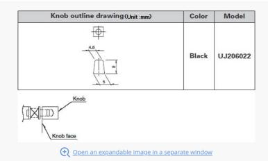
We recommend the use of adhesive to secure the knob when mounting onto switches.
